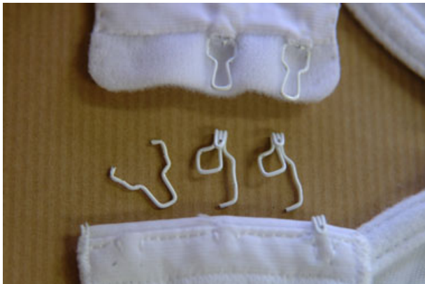
FIG. 5—Damaged hooks, eyes, and bra fabric as a result of considerable force in an attempt to pull the bra off the wearer.
