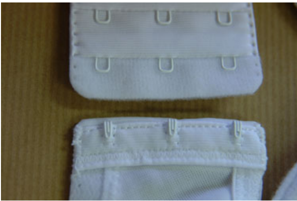
FIG. 2—Bra hooks and eyes stitched in position.
