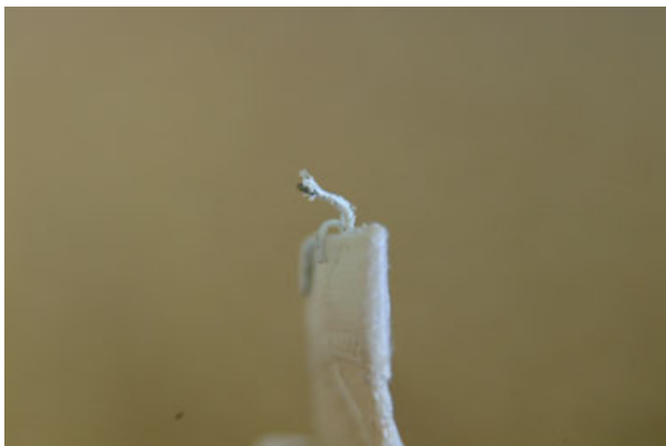
FIG. 6—Damage to bra hook by washing machine.
